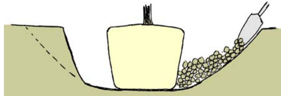
Figure 8. When dug with an auger, cut down the sides into the saucer shape during backfill process.
